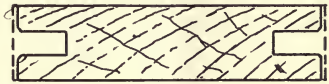
A-Showing 3" exposure after jointing and grooving stock only 3\frac{1}{4} " wide in the rough.
